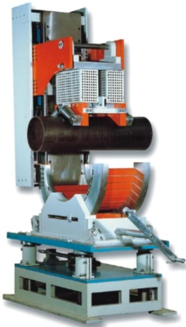
A swivelling and balancing mechanism houses a magnetic yoke and segment test head for inspection of weld line for a steel pipe.
