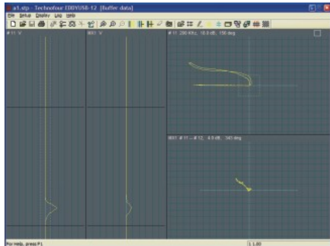
Lift-off signals can be mixed out using two frequencies, simplifying surface crack detection
