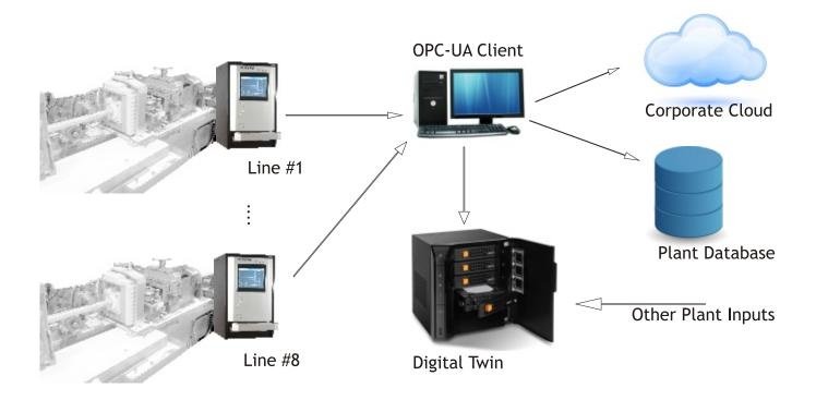
**TECHNOFOUR GX systems** implement an integral OPC-UA server listening on port 4840. The server can accept connections from one or more OPC-UA clients on local network. Several tags are defined on the server. These tags are of type string, integer and arrays of integers. Clients can subscribe to these tags and receive updated values as and when available. Servers are implicitly located in a secure environment, and only implement anonymous logins.
