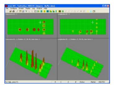
Technofour ViRAT array probes can be used with INSIS-EX for detection of tight cracks like PWSCC in tubesheet area, roll-transition regions and Ubends. ViRAT offers significant improvement over motorized pancake probes in terms of speed of inspection, costs and reliability. 3D C-Scans present eddy current data for a more intuitive recognition of defects. Any indication can be analyzed in a corresponding 2D display using familiar phase analysis against calibration curves.
